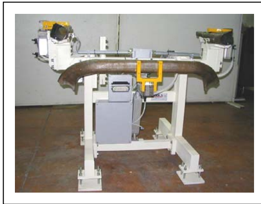
PARTICULAR CAR AXLE PREDISPOSITION FOR ROBOTIZED PLASMA ARC CUTTING
