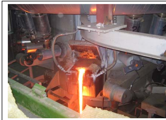
MELT SECTION ROCKWOOL PRODUCTION PLANT
