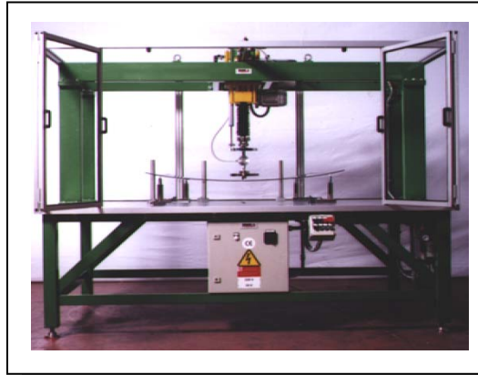
GLASS TEST BENCH BREAKING LOAD CONTROL AND MAXIMUM DEFLECTION
