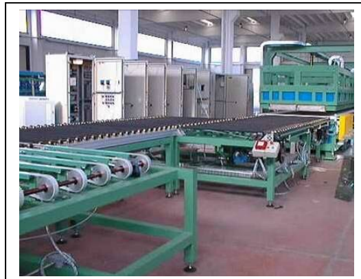
LOAD FURNACE SECTION WITH TERMOREGULATION CONTROLLED BY P.L.C.
